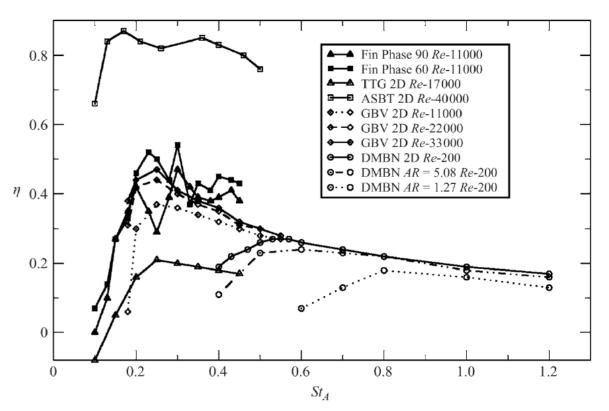
• <u>Optimization target</u>: St = 0.3 (maximum swimming efficiency for most of fishes)
